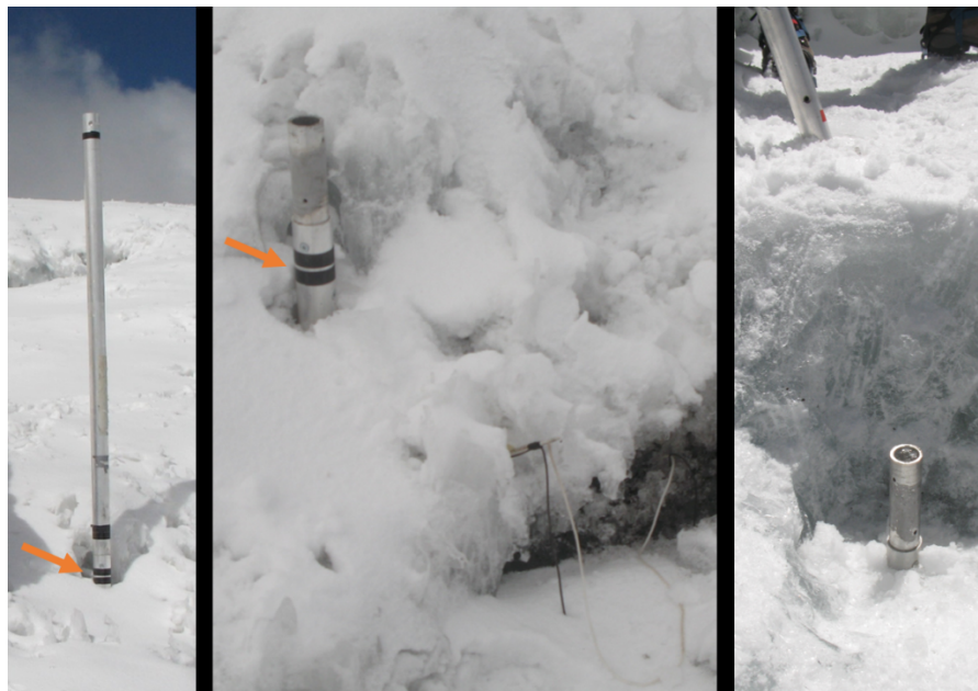
Figure 6 Pictures from September 2009 (by M. Winkler) showing the segments of the temperature string tower (left and center) and the AWS3 (right) that had to stay in the ice. The spare part of the temperature string tower (left) was recycled when redrilling AWS3. Remnants of the temperature string sensors can be seen in the center picture. The arrows point to the two black tapes, that led to secure identification of the segments in 2023 (see Figure 10).
