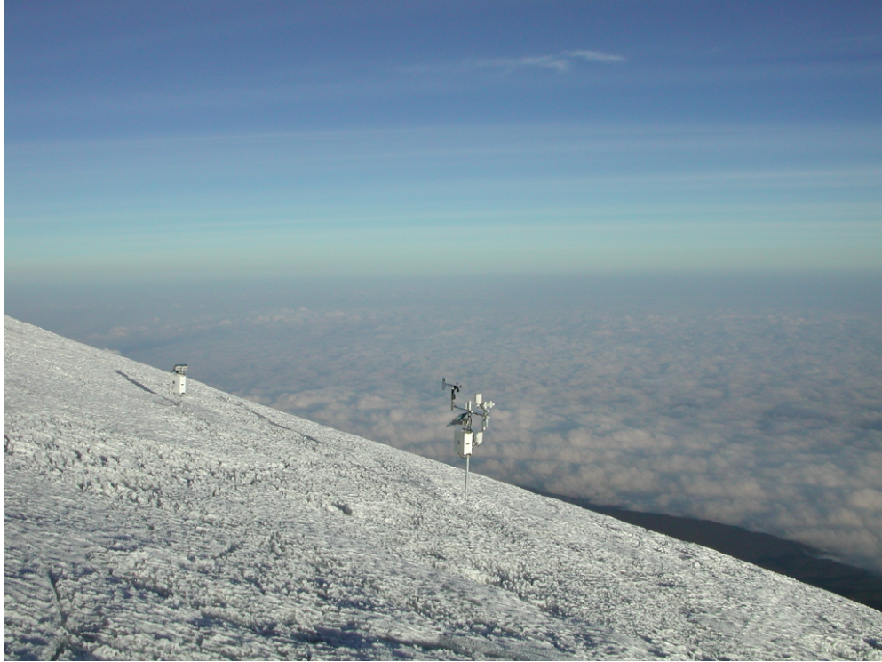
Figure 5 AWS3 on the uppermost part of Kersten Glacier (installed on February 8 th , 2005) at 5873m and a mast tower with a temperature string about 10 meters to the East of it. The latter was installed in July 2005, and it was set out of order and detached (except the mast) before 2008. The picture was taken by N. Cullen in July 2005.
