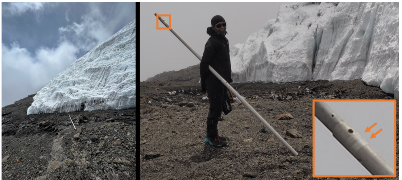
Figure 10 E. Collier found the two mast segments of the temperature string tower that had to remain in the ice. The place of discovery was the lower (Southeastern) edge of the upper remnant of the Kersten Glacier (point (C) in Fig. 2). The arrows mark the tape traces that led to identification (cf. Figure 6; left and center). The picture was taken by M. Winkler on October 4 th , 2023.
