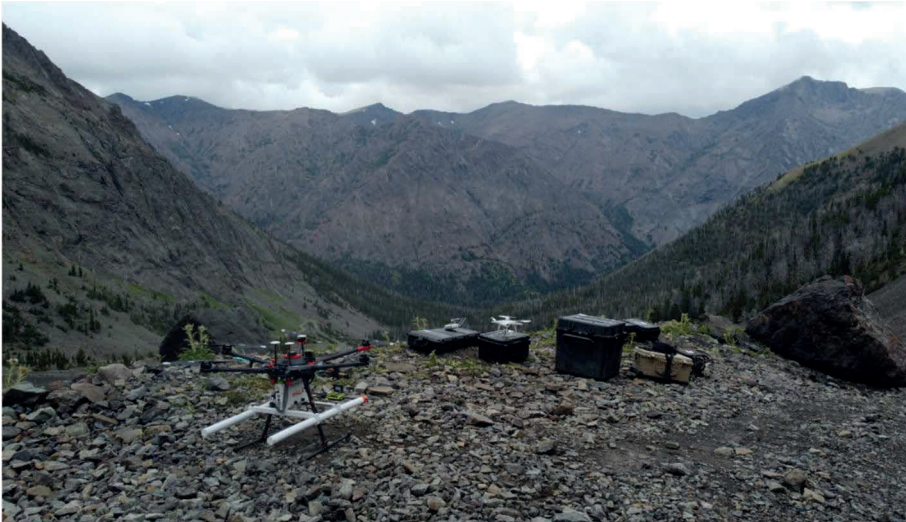
Figure 2: A drone-mounted Malå ground penetrating radar system and DJI Phantom 4 at Galena Creek rock glacier, Shoshone National Forest, Wyoming. The Malå drone flies at a constant elevation (1 m) above the rock glacier surface to collect information about the debris-ice interface depth. Photo: Daniel Thomas
