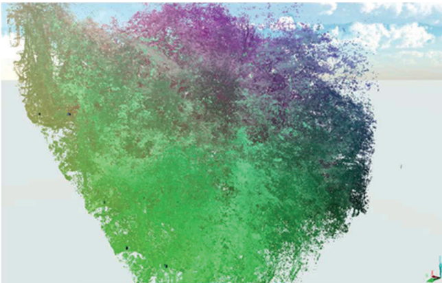
Figure 2: Point cloud of a 25 x 25 m 2 forest parcel on the hillside of mount Agou, Togo, colored according to x, y, and z-axis. The small boxes on the left side show scan positions of a FARO M70 terrestrial laser scanner. The same forest was also sensed with a LiDAR and multispectral UAV to allow future data fusion.
