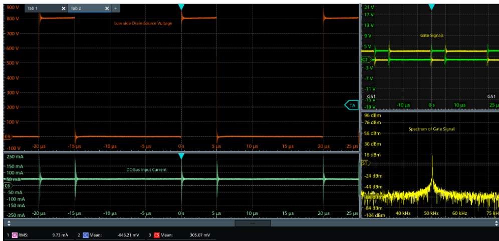
Half Bridge Constant Duty Operation Test
