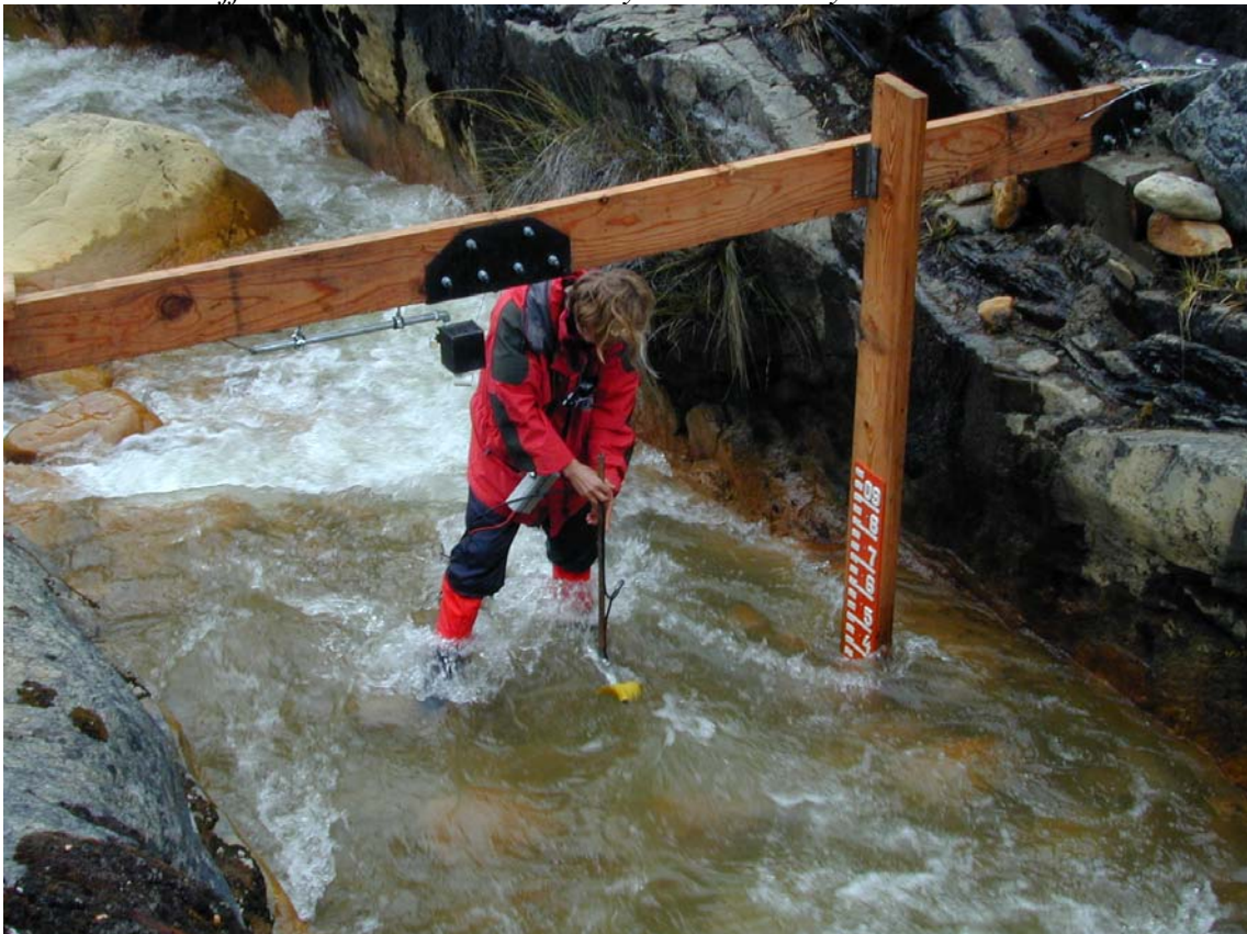
Figure C.19: Calibration measurement at the runoff station at Glacier Chinchey (4200 m a.s.l.). Photo taken by Georg Kaser in November 2001.
