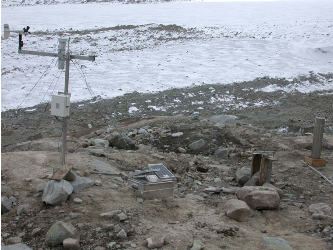
Figure C.9: AWS-south at Glacier Artesonraju (4850 m a.s.l.) with a precipitation gauge. Photo taken by Irmgard Juen in July 2004.
