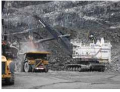
Figure 9: Loading of a haul truck wish freshly blasted ore.
