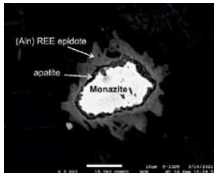
Fig. 1B Monazite breakdown into coronas of apatite and allanite in the S-type granite (Tribeč Mts. Fatric Unit). BSE image.
